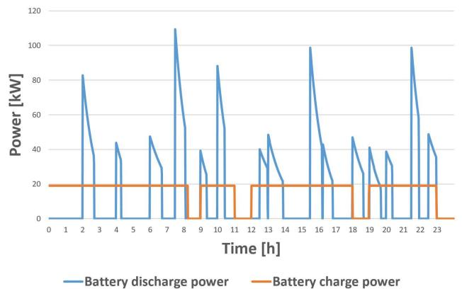
Figure 1 Battery charge and discharge power – Location I
