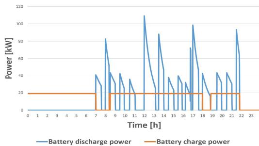
Figure 6 Battery charge and discharge power – Location II 2030
